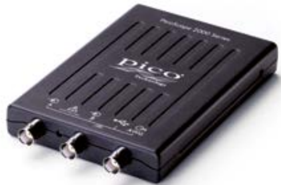
2-channel oscilloscope: 2204A and 2205A
